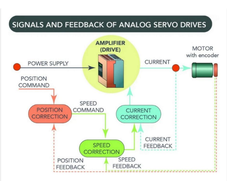
Unlike digital servo drives, analog types have no processing ability — that is, no ability to make computations in the drive. This is actually a benefit in terms of servo response time, because the system doesn't spend time waiting for a digital processor to make the necessary computations and determine the response.
